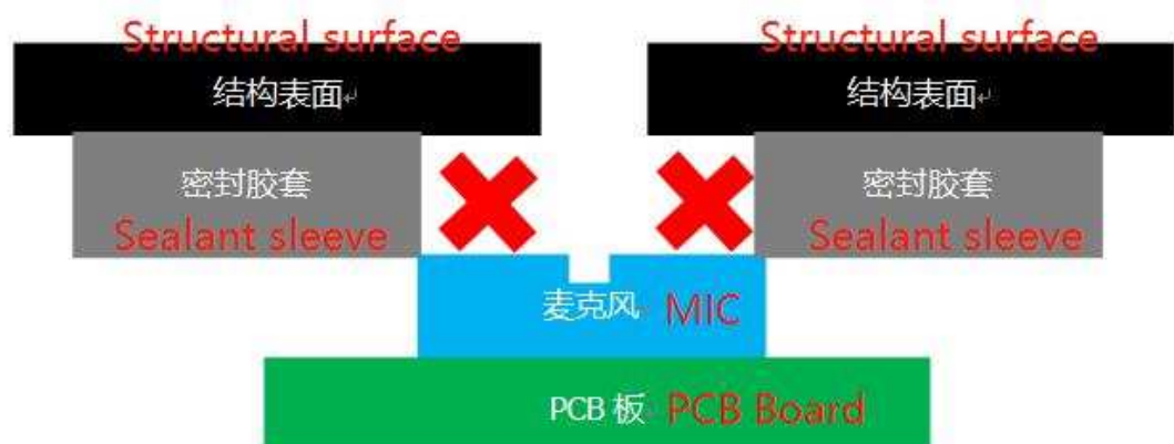
Fig5 TOP Helmholtz resonator
