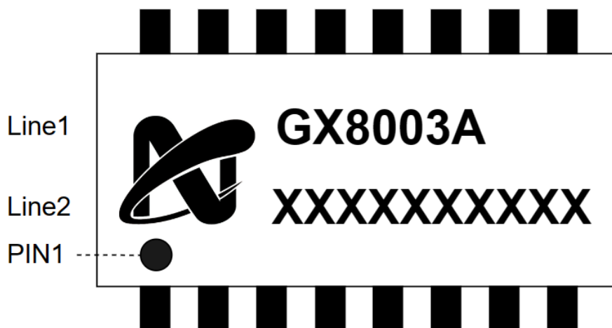
Figure 7-2 Chip mark description
